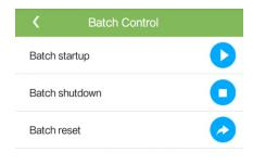
**Step 3** Tap **Batch startup**, **Batch shutdown**, or **Batch reset**, enter the password for logging in to the app, and tap **OK**.
