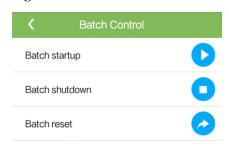
**Step 3** Tap **Batch startup**, **Batch shutdown**, or **Batch reset**, enter the password for logging in to the app, and tap **OK**.
