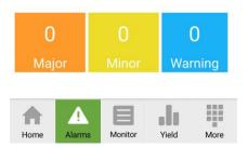
Step 2 To query the detailed alarms of an alarm severity, tap Major, Minor, or Warning.
