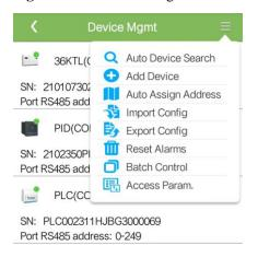
Step 2 Tap Reset Alarms, and select devices on the Reset Alarms screen.
